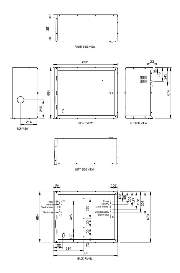
Figure 2-4: Vortex Eco External and External System 12/16 and 16/21
