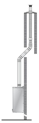
Figure 9-4: Green to Orange flue system
