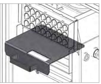
Figure 4-4: Removing baffles from boiler shell
