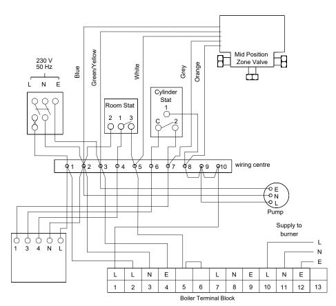
Figure 8-2: External wall hung - 3-port valve control system
