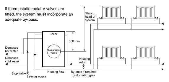
Figure 7-2: Sealed system boilers
