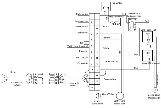
Figure 8-5: External wall hung - wiring diagram
