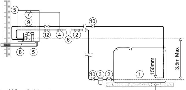
Figure 3-3: De-aeration device system
