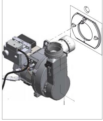
Figure 3-5: Burner removal
