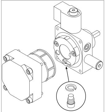
Figure 3-6: Fitting/location of 'hoseshoe' washer
