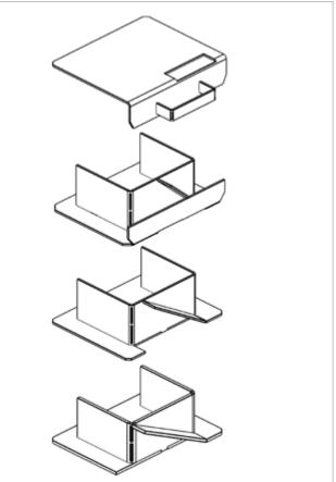
Figure 4-6: Re-fitting baffles into boiler shell
