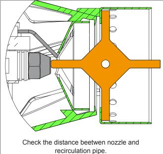
Figure 10-5: Checking the diffuser position using the guage provided
