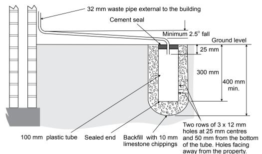
Figure 6-1: Purpose made condensate soakaway
