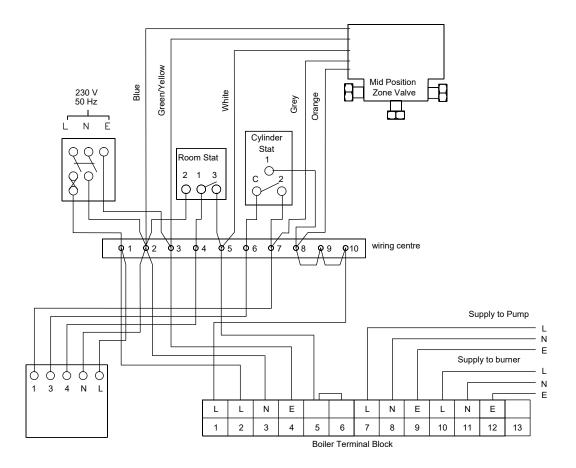
Figure 8-4: External system wall hung - 3-port valve control system Section 8: Electrical
