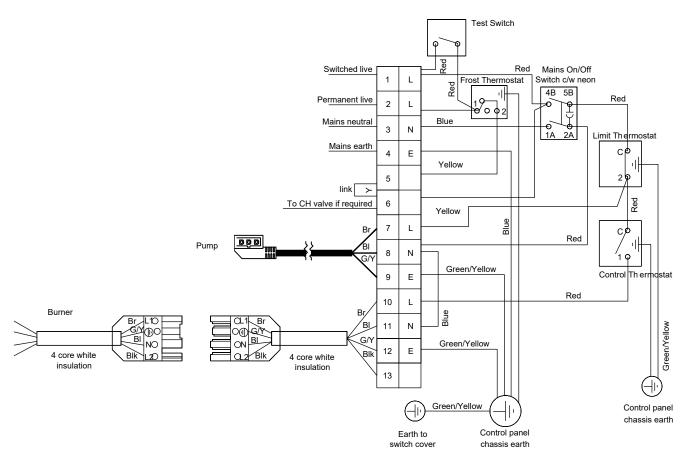
Figure 8-6: External system wall hung - wiring diagram
