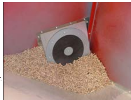
Figure 2-1: Contents switch in the base of the
