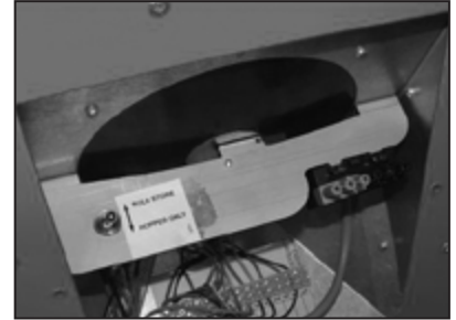
Figure 8-1: Hopper selector switch and 6-way plug
