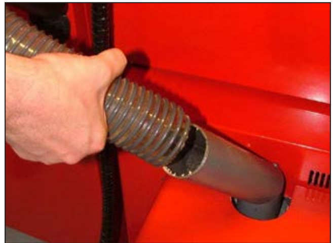
Figure 10-3: Disconnect pellet hose from burner
