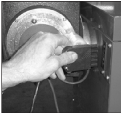
Figure 11-1: Disconnecting hopper 5-way plug
