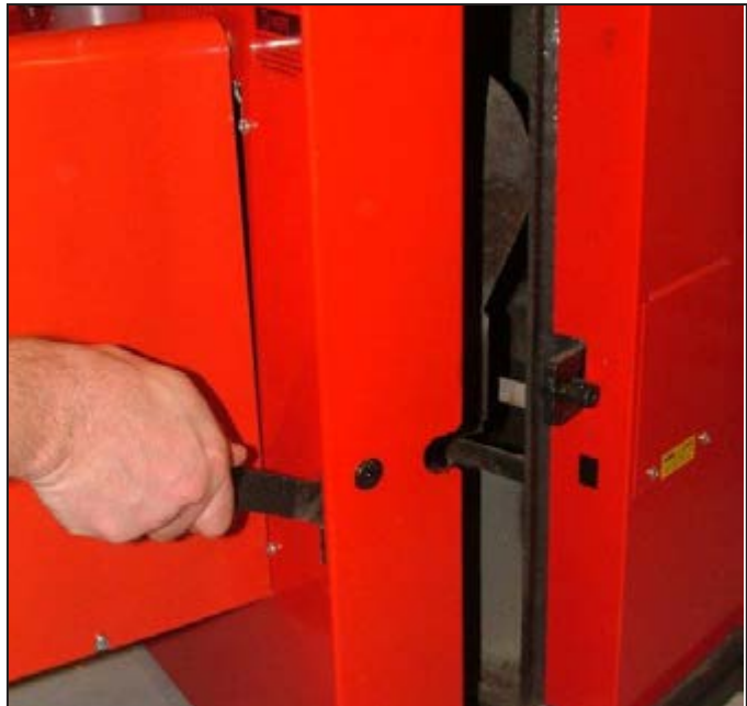
Figure 10-5: Opening combustion chamber door
