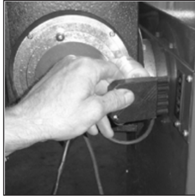
Figure 8-3: Hopper plug connection
