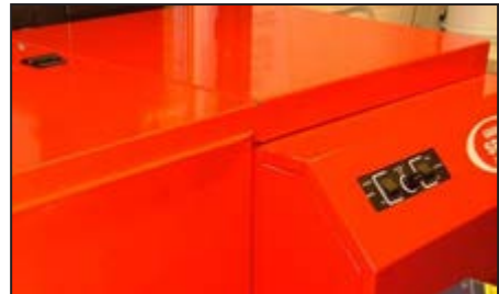
Figure 7-5: Correct alignment of hopper to boiler.
