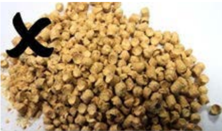
Figure 3-4: Pellets too short in length
