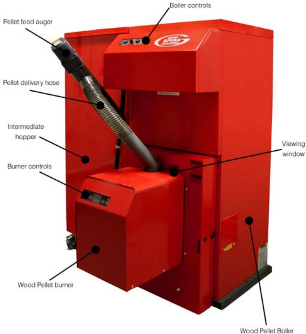
Figure 1-1: Grant Spira Condensing Wood Pellet Boiler and Intermediate Hopper
