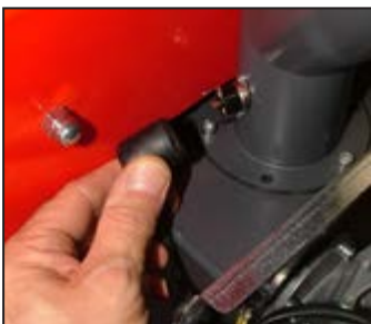
Figure 10-6: Removal of thermostat lead
