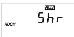
The control is no longer able to read the indoor sensor due to a short circuit. The control will continue to operate as if there was nothing connected to the indoor sensor input. Locate and repair the problem as described in the GEO 360 Sensors Data Brochure. To clear the error message from the control after the sensor has been repaired, press the **Item** button.
