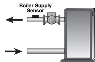
**Note:** The boiler pump should not be operated by the boiler's thermostat, as this may lead to improper cycling of the boiler because of inconsistent flow past the boiler supply sensor.
