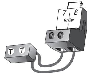
**⚠ Sensor and Unpowered Input Connections**
