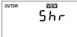
The control is no longer able to read the outdoor sensor due to a short circuit. In this case the control assumes an outdoor temperature of 0°C and continues operation. Locate and repair the problem as described in the GEO 360 Sensors Data Brochure. To clear the error message from the control after the sensor has been repaired, press the **Item** button.
