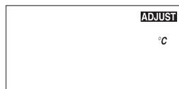
Press and release the **Item** button to advance to the units adjustment. Use the ▲ or ▼ button to set the scale to °C or °F.
