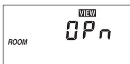
The control is no longer able to read the indoor sensor due to an open circuit. The control will continue to operate as if there was nothing connected to the indoor sensor input. Locate and repair the problem as described in the GEO 360 Sensors Data Brochure. If the indoor sensor is deliberately removed, the control must be powered down, and then powered back up. To clear the error message from the control after the sensor has been repaired, press the **Item** button.
