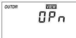
The control is no longer able to read the outdoor sensor due to an open circuit. In this case the control assumes an outdoor temperature of 0°C and continues operation. Locate and repair the problem as described in the GEO 360 Sensors Data Brochure. To clear the error message from the control after the sensor has been repaired, press the **Item** button.
