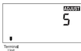
Press and release the **Item** button to advance to the *terminal unit (heat emitter)* adjustment. Use the ▲ or ▼ button to select the desired terminal unit (heat emitter). The terminal unit (heat emitter) number corresponds to the type of terminal that is being used. The table below lists the terminal units (heat emitters) and their default values.
