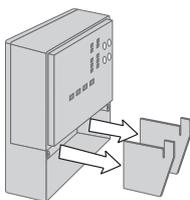
Remove the safety dividers from the wiring chamber by pulling them straight out of their grooves.
