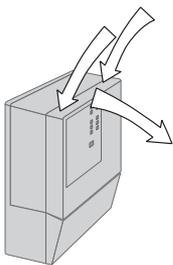
Press down at the fingertip grips on top of the front cover and pull out and down.
