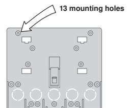
The base is ready for mounting. There are 10 conduit knock-outs at the back and bottom of the wiring chamber.
