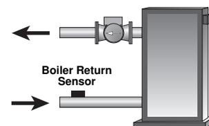
**Note:** The boiler pump should not be operated by the boiler's thermostat, as this may lead to improper cycling of the boiler because of inconsistent flow past the boiler return sensor.
