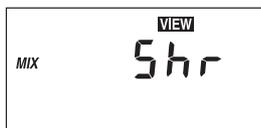
The control is no longer able to read the mixing supply sensor due to a short circuit. In this case the control will operate the mixing valve at a fixed output as long as there is a mixing demand. Locate and repair the problem as described in the GEO 360 Sensors Data Brochure. To clear the error message from the control after the sensor has been repaired, press the **Item** button.
