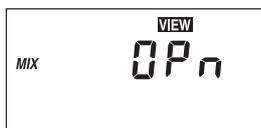
The control is no longer able to read the mixing supply sensor due to an open circuit. In this case the control will operate the mixing valve at a fixed output as long as there is a mixing demand. Locate and repair the problem as described in the GEO 360 Sensors Data Brochure. To clear the error message from the control after the sensor has been repaired, press the **Item** button.
