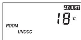
Press and release the **Item** button to advance to the ROOM UNOCC adjustment. Use the ▲ or ▼ button to set the desired temperature. The ROOM UNOCC setting is set to the desired room air temperature during the unoccupied (Night) mode.
