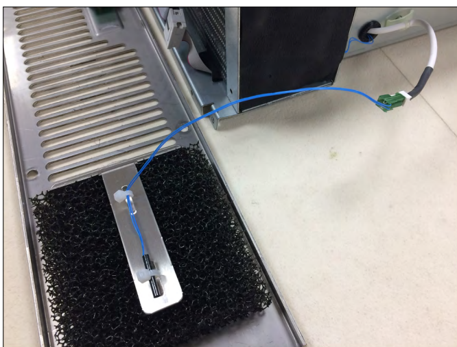
Figure 3-8: Solo Hideaway air temperature sensor and plug
