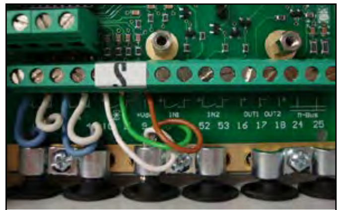
Figure 7-16: User sticker seal over flow meter connections
