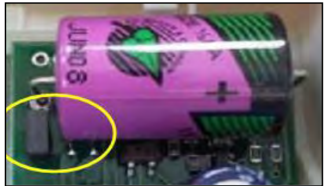
Figure 7-21: Back-up battery with jumper fitted
