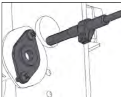
Figure 8-4: Removing the photocell
