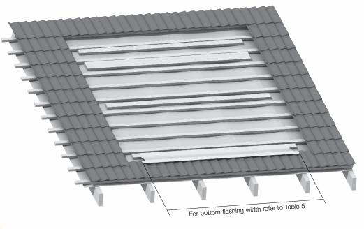
Mark position of both ends of bottom flashing on batten. Remove left hand flashing and fix right hand flashing to batten using suitable small screws (not supplied).
