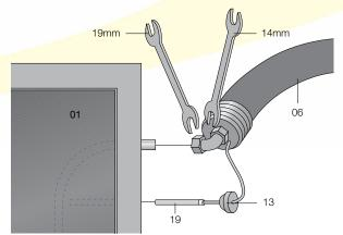
Figure 91: Connection of Temperature Sensor
