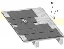
Figure 32: Fixing Mounting Battens and Roof Anchors through Sarking
