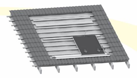
Figure 56a: Installation of Lower Base Tray
