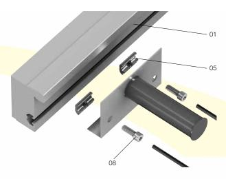
Figure 81: Fixing the Carry Handles
