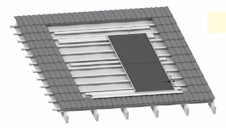
Figure 56b: Installation of Upper Base Tray
