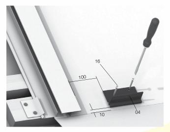
Figure 67: Fixing of bottom Mounting Brackets
