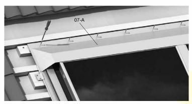
Figure 73: Fixing left hand Top Cover Flashing (07-A)
