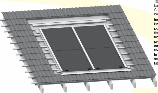
Figure 66: Location of bottom Mounting Brackets
