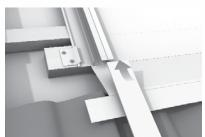
Figure 64: Installation of Cover Sheets
