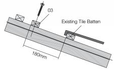
Figure 52: Bottom Fixing Batten
