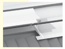
**Figure 55:** Installation of Additional Bottom Flashings
