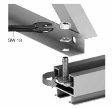
Figure 41: Fixing Using Interlocking Bolt
