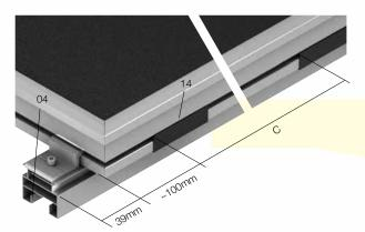
Figure 82: Positioning the Mounting Hooks
