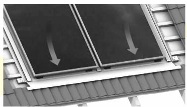
Figure 69: Installation of the Collectors on to Bracket
