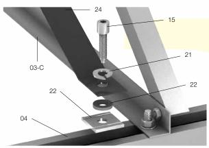
Figure 45: Fixing the Securing Cruciform and Mounting Rail
