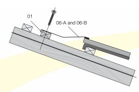
**Figure 54:** Installation of Bottom Flashing
