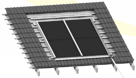
Figure 62: Fitting of Cover Strips
