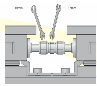
Figure 88: Hydraulic Connection
