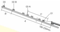
Figure 53: Top, Upper middle, Lower middle and Bottom Horizontal Fixing Battens
