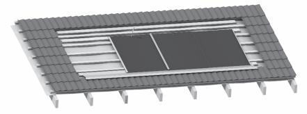
Figure 58c: Installation of Third Tray
