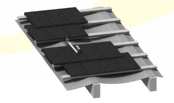
Figure 28: Fixing Mounting Battens and Roof Anchors
