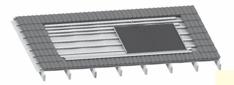
Figure 58b: Installation of Second Tray
