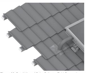
Figure 98: Detail View of Solar Collector Field Connection - On-Roof Systems
