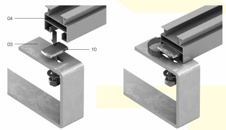
Figure 34: Fixing the Mounting Rail
