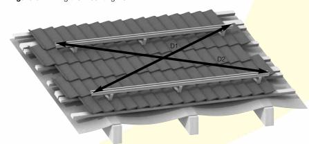
Figure 35: Aligning the Mounting Rail
