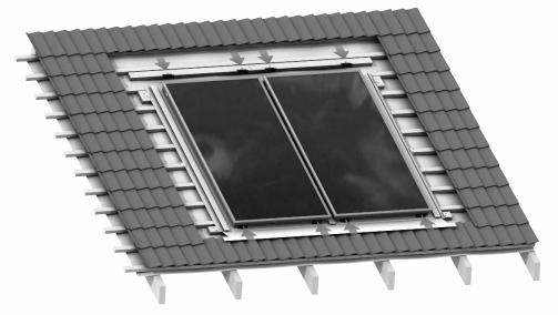
Figure 70: Installation of the Top Brackets
