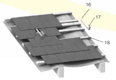
**Figure 31:** Fixing Mounting Battens and Roof Anchors
