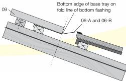
Figure 56c: Section Through Bottom Flashing
