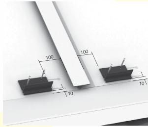
Figure 68: Bottom Mounting Bracket Dimensions
