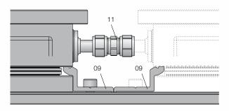
Figure 85: Align Anchor Block for Additional Fixing Brackets
