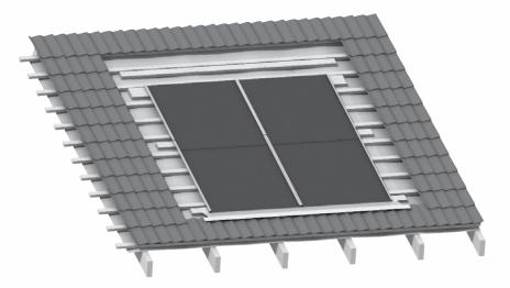
Figure 57b: Installation of Second Base Tray
