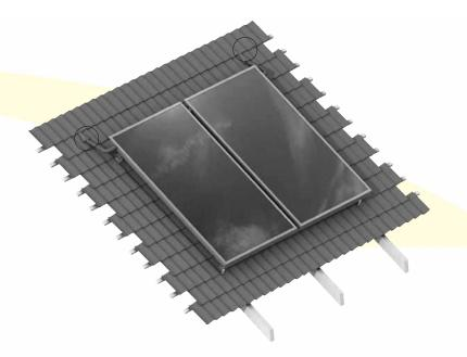
**Figure 93:** Solar Collector Field Attachment for On-Roof Systems
