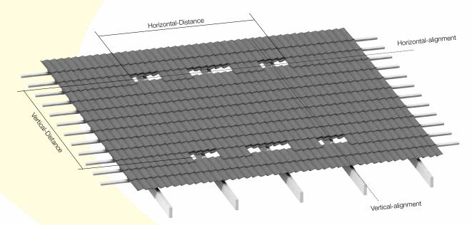
Figure 24: Horizontal and Vertical Alignment
