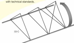
**Figure 46:** Fixing Additional Flat Roof Mounting Brackets
