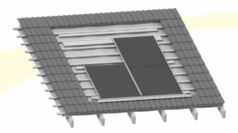
Figure 57a: Installation of First Base Tray
