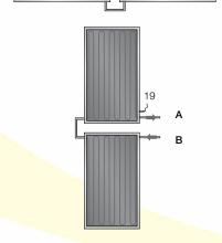
**Figure 79:** Connections for Two Portrait Format Collectors Mounted one Above the Other
