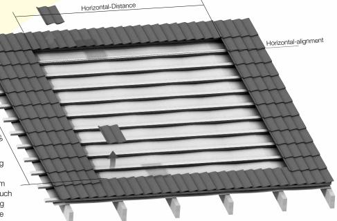
Figure 50: Remove Roof Covering
