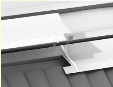
Figure 55: Installation of Additional Bottom Flashings
