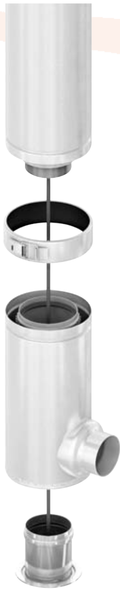
a) Boiler to rigid flue connection
