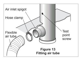
Remove the test point screw.
