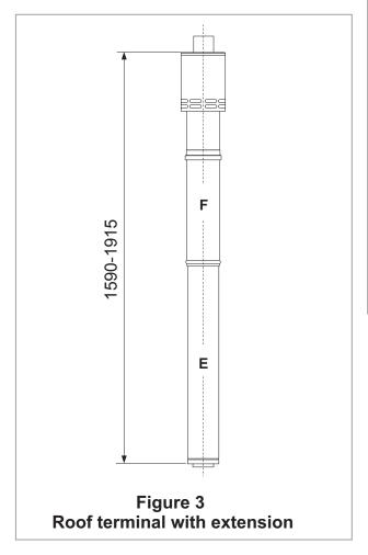
Sections (C) and (D) combine to form a telescopic length. Terminal section (F) slides telescopically over fixed length section (E).
