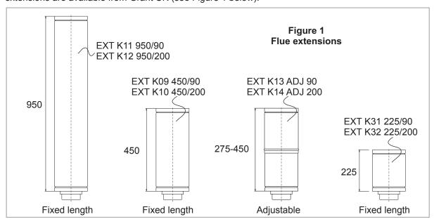
The dimensions shown are measured from the top of the boiler flue outlet, on cased models. The distance between the boiler flue outlet and the top of the casing should be taken into consideration.
