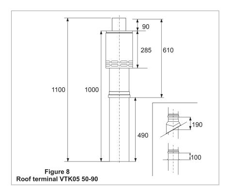
**Note:** The position of the storm collar. The storm collar locates into the top of the Grant pitched and flat flashing.
