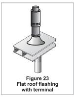
Fit the terminal section (F) ensuring that the integral storm collar locates correctly over the flashing. The terminal section slides telescopically over the section below it (except when fitted to section (D), fit the bracket ensuring that the weight of the terminal is carried by the clamp supplied and not by the flashing.
