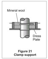
If required fit the fire stop kit as shown in Figures 16 to 21. Construct a boxing as shown. Fill the void around the flue pipe with rockwool or glassfibre insulation.
