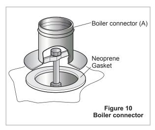
Locate the boiler connector (A) centrally into the gasket on the top of the boiler. Tighten the bolt to fix the connector in place (see figure 10).
